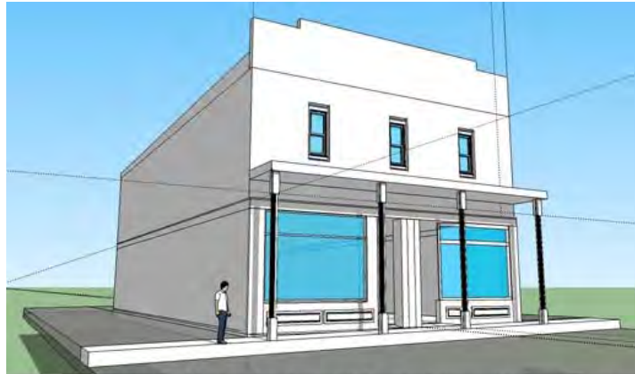
High Verandah – Made of substantial materials and turned posts
